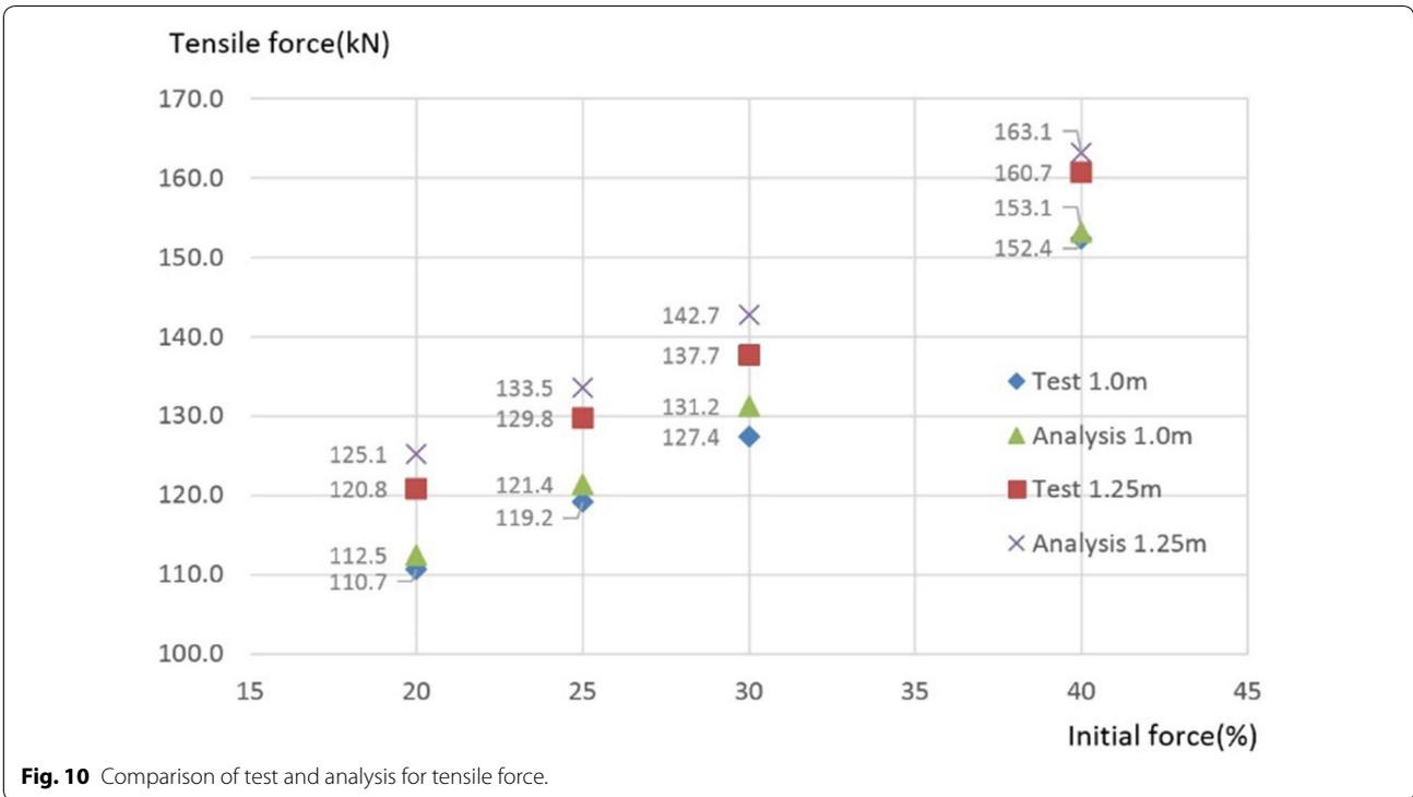
**Fig. 10** Comparison of test and analysis for tensile force.
