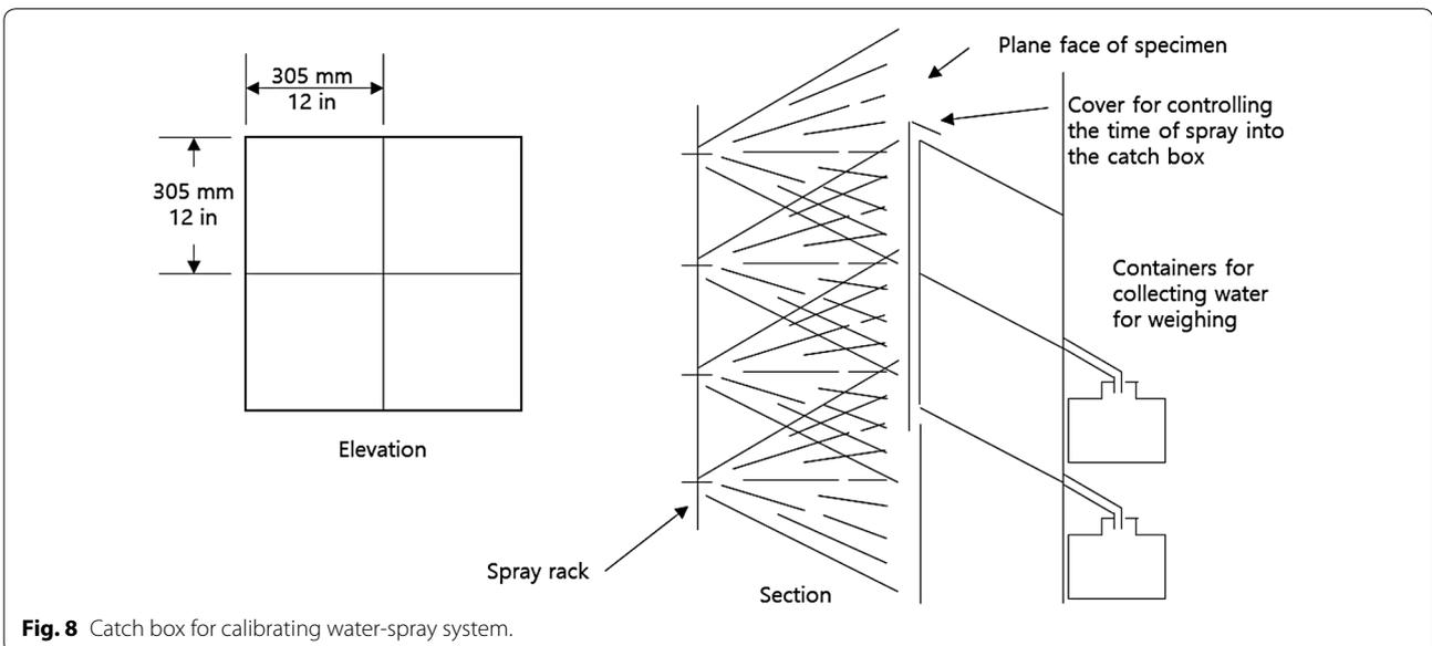
**Fig. 8** Catch box for calibrating water-spray system.
