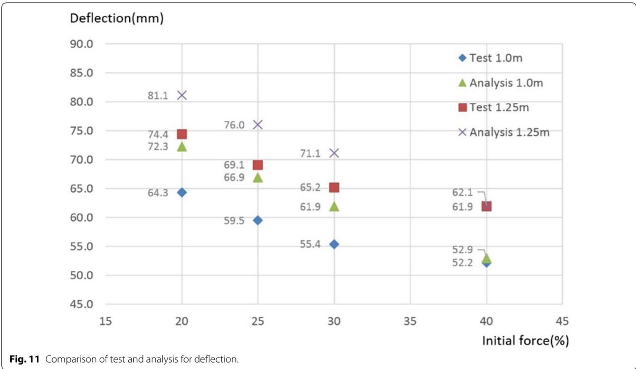
**Fig. 11** Comparison of test and analysis for deflection.
