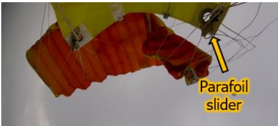
Figure 24 Twisted line due to parafoil slider
