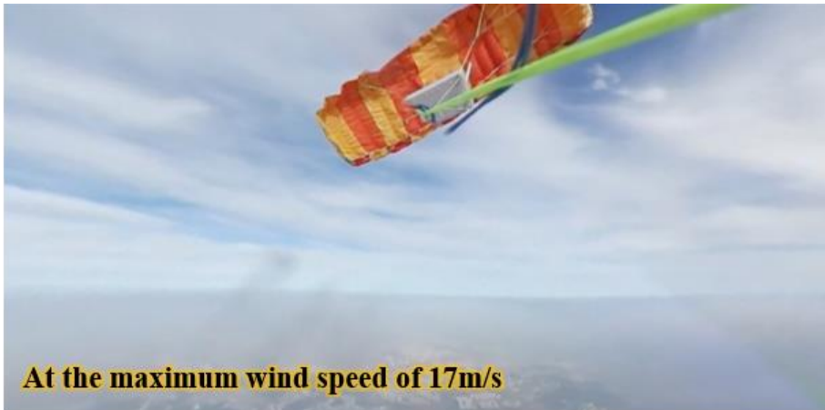
Figure 27 The influence of the wind on the parafoil
