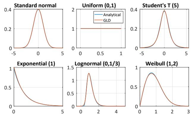
Figure 1: Some parametric PDFs approximated using the generalized lambda distribution.
