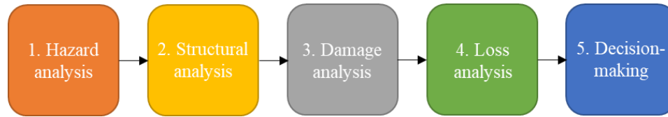
Figure 1. Steps in the performance-based framework for evaluating building performance.
