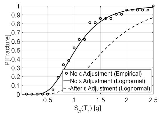
Figure 2: An example of  $\epsilon$  adjustment for fracture fragility curves subjected to far-field ground motions
