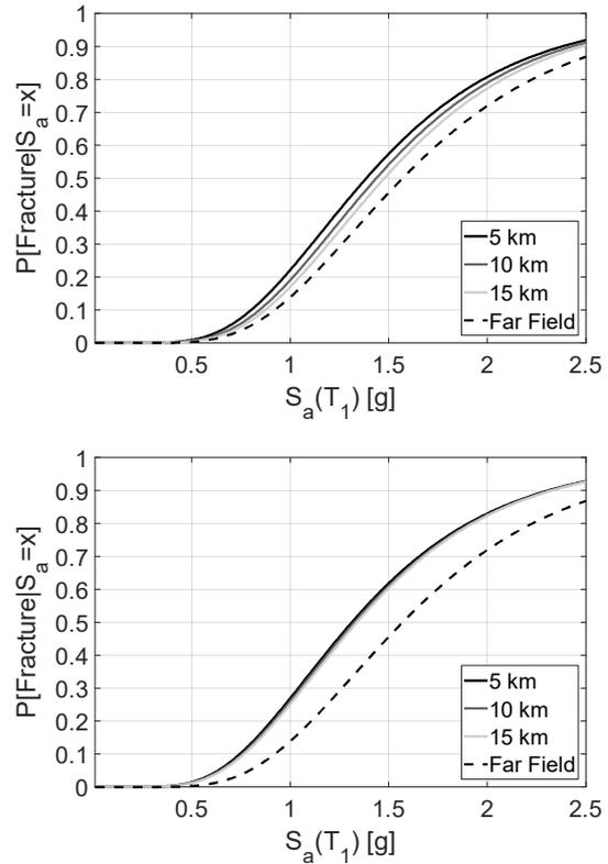
Figure 5: Fracture fragility functions for 4-story frame at three different midfault (top) and end-of-fault (bottom) sites, with far-field fragility curves
