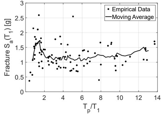
Figure 3: Relationship between fracture  $S_a(T_1)$  of 4-story frame and  $T_p/T_1$  ratio of 91 pulse-like records
