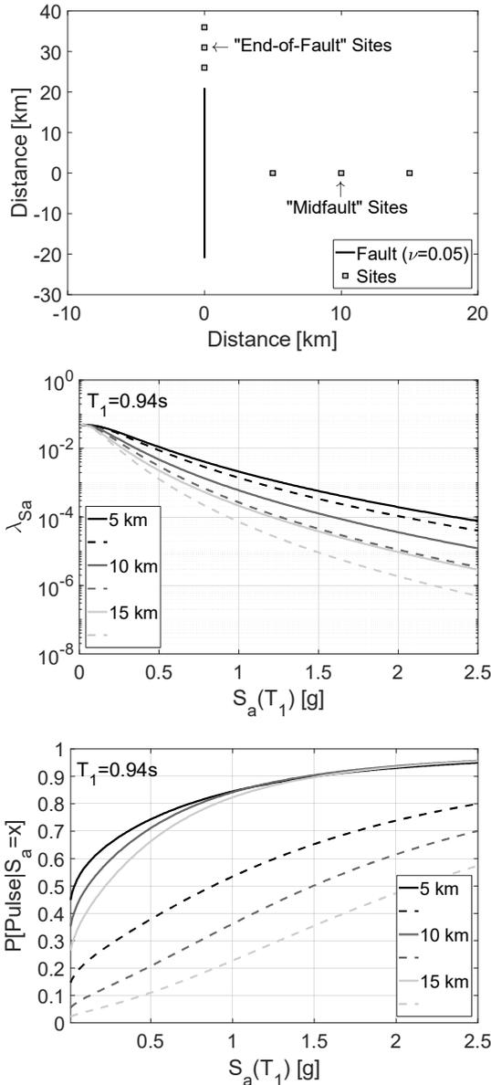
Figure 4: Representative near-fault sites considered, showing site locations (top); results of seismic hazard curves (middle) and probabilities of pulse occurrence (bottom) for 4-story frame ( $T_1 = 0.94$  s) at midfault (dashed lines) and end-of-fault (solid lines) sites
