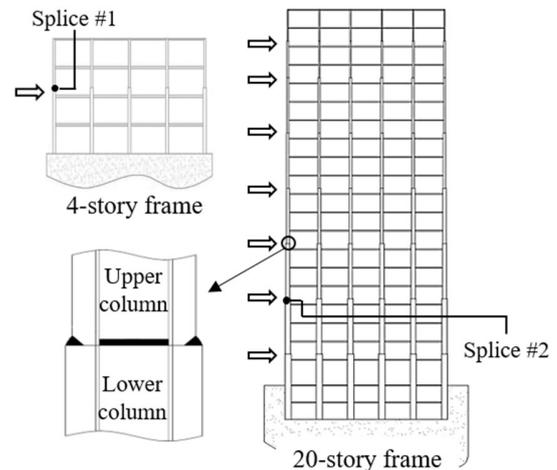
Figure 1: Schematic illustration of 4-story and 20-story steel frame models and welded column splice
