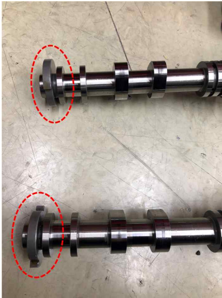
Figure 3.8 Camshaft and the 'half moon' part
