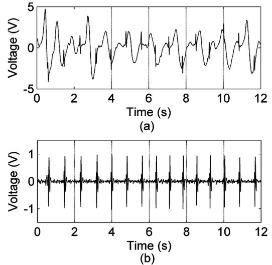
Fig. 7. ECG recording obtained with the subject swinging the upper body back and forth, wearing a regular woolen business suit, (a) 0.5 Hz~35 Hz, (b) 8 Hz~35 Hz.
