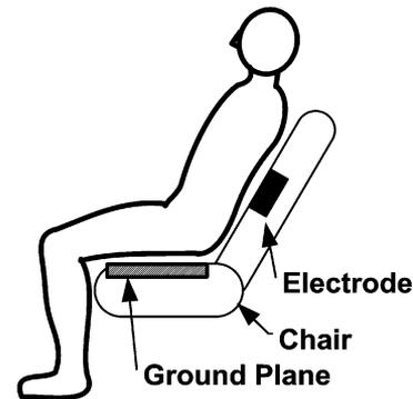
Fig. 1. Experiment setup used for ECG measurements using electrodes located on a chair.
