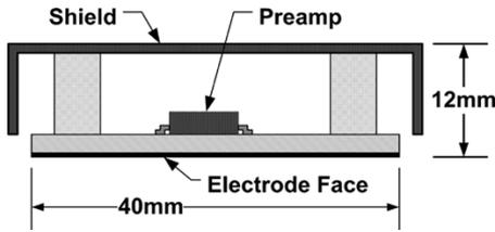
Fig. 4. Configuration of the active electrode.
