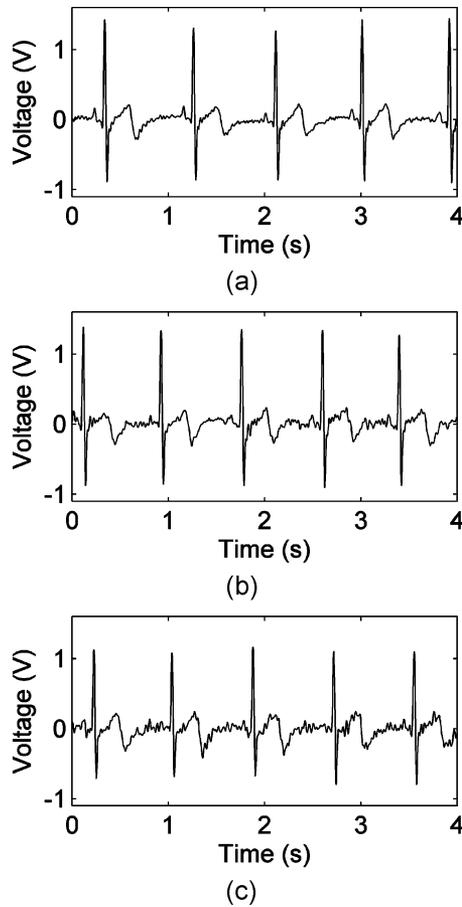
Fig. 5. ECG waveforms obtained by the presented method; (a) through a cotton shirt (twill weave, thickness 0.33 mm), (b) through a woolen business suit (thickness 0.37 mm) over a cotton dress shirt (thickness 0.22 mm), and (c) through an acrylic shirt (twill weave, thickness 0.65 mm). In all cases, the subject wore cotton underwear. Thickness gauge: Mitutoyo 7301.
