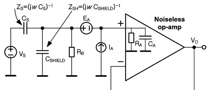
Fig. 2. Diagram of the amplifier used with an indirect-contact electrode ( $C_S$ ) and signal source (ECG source,  $V_s$ ).
