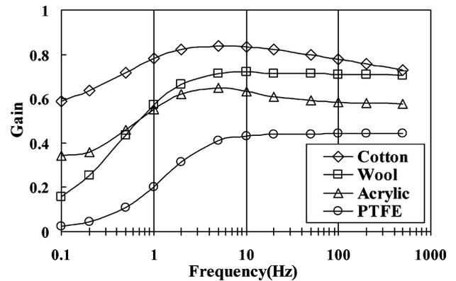
Fig. 8. Frequency responses of the active electrode for different types of clothing and for a PTFE plate: cotton (twill weave, thickness 0.6 mm), wool (twill weave, thickness 0.55 mm), acrylic (twill weave, thickness 0.65 mm), and PTFE plate (thickness 1.5 mm, relative permittivity 2).
