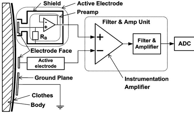
Fig. 3. Block diagram of the indirect contact ECG measurement.
