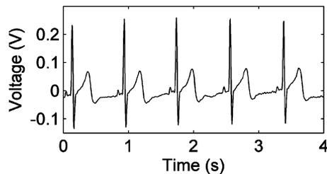
Fig. 6. ECG waveform obtained with conventional Ag-AgCl electrodes attached to the back skin of the same subject as in Fig. 5 (BIOPAC MP150, gain 1000, 0.5 Hz~35 Hz).
