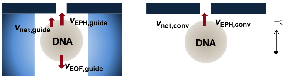
Figure 2–18 Velocity contributions to a translocating DNA in the nanopores. The velocity terms explained in the text and their directions are marked on 1 kbp dsDNA molecules (gray circles) approaching the sensing layer in the guide–inserted (left) and the conventional (right) nanopore devices. The images are not in scale. Figures were from ref. 1 - Adapted by permission of the Royal Society of Chemistry.
