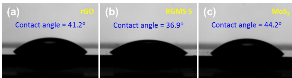
Figure 3.5. Surface tension of water drops on (a) rGO, (b) RGMS 5 and (c) MoS 2 .
