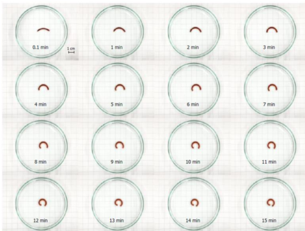
Figure IV-9. Time-lapsed photographs of the bending of the hydrogel bilayer in a pH 7 buffer solution at 25 °C.
