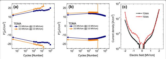
Fig. 5 The results of endurance test of (a) TEMA HZO (reproduced from Ref. 39) and (b) TDMA HZO with the electric field cycling and pulse field amplitude of 2.5 and 3.0 MV/cm. The frequency of the rectangular double pulse for the endurance test was fixed at 100 kHz. (c) The current density–electric field curves of TDMA HZO (black) and TEMA HZO (red; reproduced from Ref. [39])
