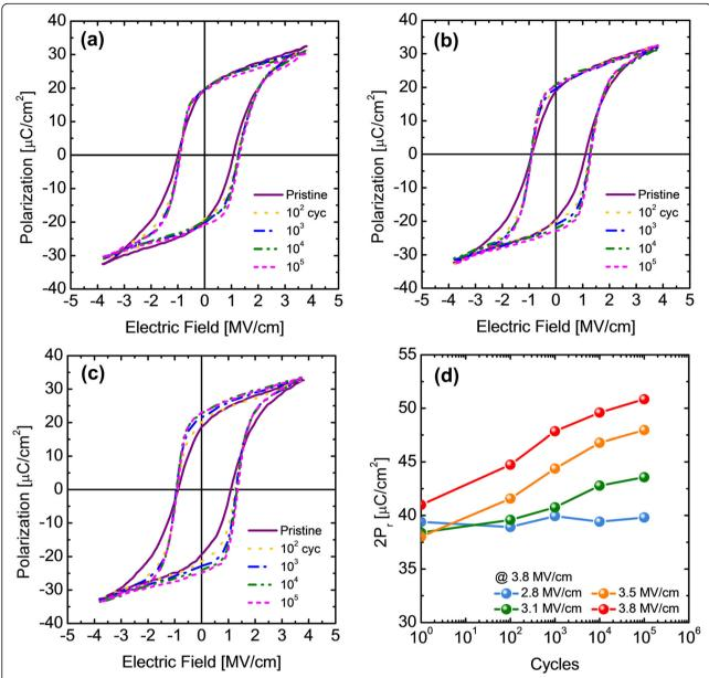
**Fig. 4** The polarization–electric field (P–E) curves measured during wake-up test with the fatigue pulse height of (**a**) 2.8, (**b**) 3.1, and (**c**) 3.5 MV/cm. (**d**) The changes in 2P<sub>r</sub> value during the endurance test with 2.8, 3.1, 3.5, and 3.8 MV/cm-high fatigue pulses
