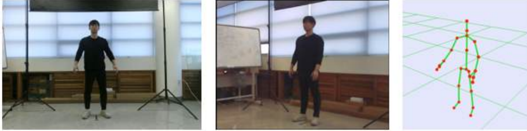
Figure 2. Sample data point from a single squat exercise. 3D keypoint data (rightmost) are actually recorded in CSV formats.
