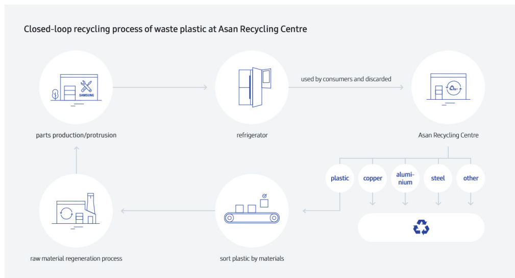
〈Figure 5〉 Samsung's Closed-Loop Recycling Process at Asan Recycling Center
