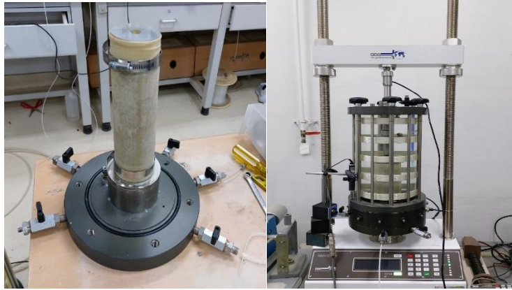
Figure. 3.2 Triaxial testing system and specimen
