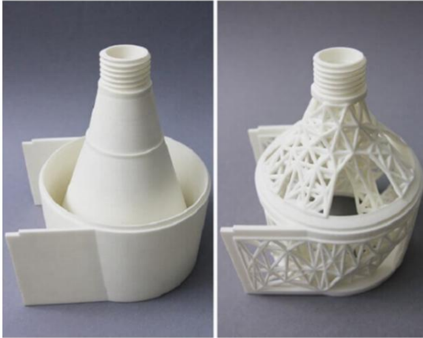
Figure 3. 3D shape with high-complexity output made using 3D printer (Right)
