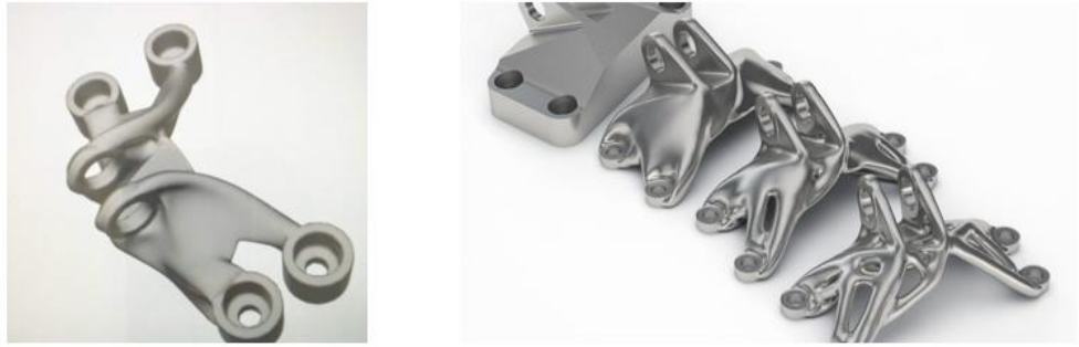
Figure 39. Result of bracket using generative design
