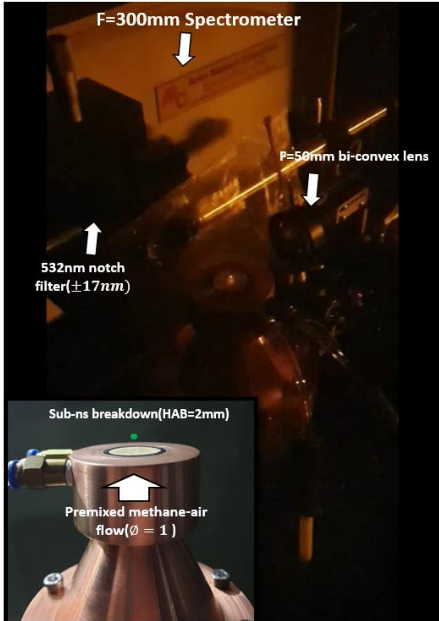
Figure 5.13 A photograph of the ps-LIBS setup. Inset illustrates the close-up image around the burner outlet.
