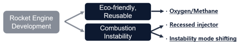
Fig. 1.4 Objectives of this study to understand the combustion instability of non-premixed flames formed by a recessed coaxial injector.
