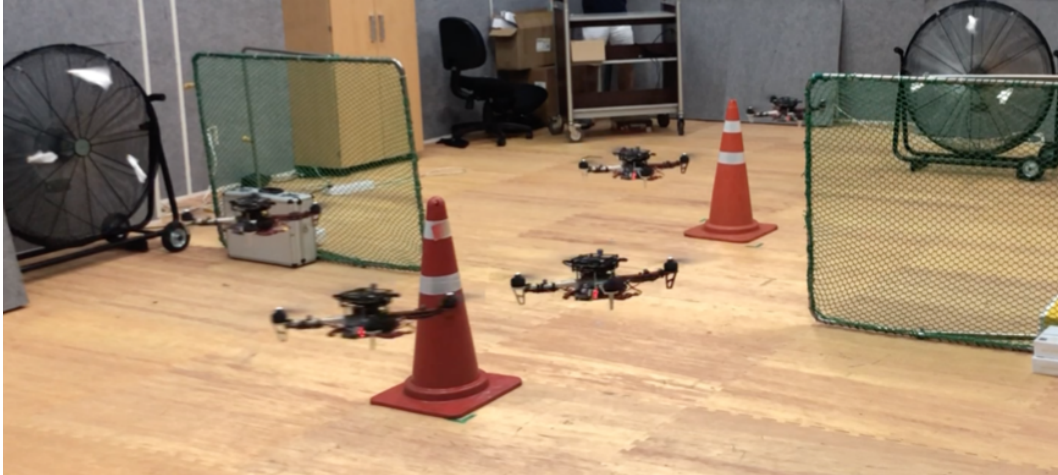
Figure 6.2: Snapshot of the experiment. Two green nets and two red cones are used as obstacles. Also, two black fans generate gusts in the environment. The multirotor avoids the obstacles against gust.
