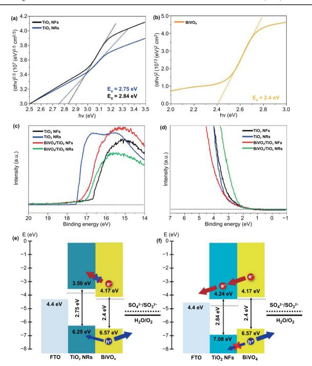
Fig. 6 UV-Vis Tauc plots of a TiO<sub>2</sub> NFs, TiO<sub>2</sub> NRs, and b BiVO<sub>4</sub>. c Secondary electron emission spectra and d valence band spectra of TiO<sub>2</sub> NFs, TiO<sub>2</sub> NRs, BiVO<sub>4</sub>/TiO<sub>2</sub> NFs, and BiVO<sub>4</sub>/TiO<sub>2</sub> NRs. Flat band structures of e BiVO<sub>4</sub>/TiO<sub>2</sub> NRs and f BiVO<sub>4</sub>/TiO<sub>2</sub> NFs
