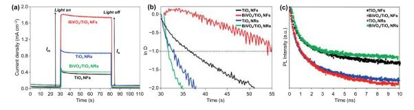
Fig. 5 a The transient photocurrent decay that occurs immediately upon illumination at 1.23 V (vs. RHE). b Transient decay times for TiO<sub>2</sub> NFs, TiO<sub>2</sub> NRs, BiVO<sub>4</sub>/TiO<sub>2</sub> NFs, and BiVO<sub>4</sub>/TiO<sub>2</sub> NRs. c TRPL of TiO<sub>2</sub> NFs, TiO<sub>2</sub> NRs, BiVO<sub>4</sub>/TiO<sub>2</sub> NFs and BiVO<sub>4</sub>/TiO<sub>2</sub> NRs
