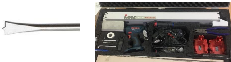
Figure 4-3 Drill resistance device (IML F500-S)
