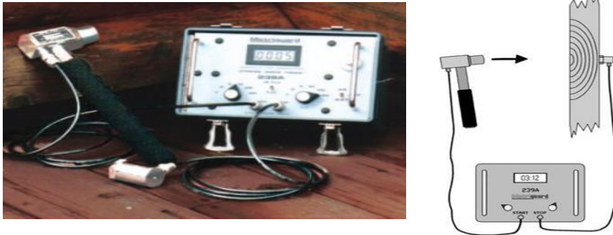
Figure 4-1 Stress wave measuring device (Metriguard 239A)
