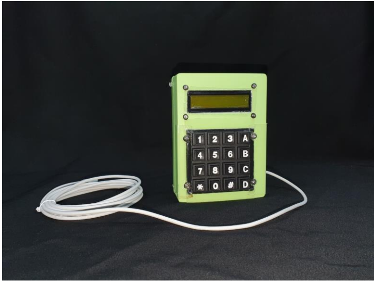
Figure 18. Credit registration module including a keypad and a display
