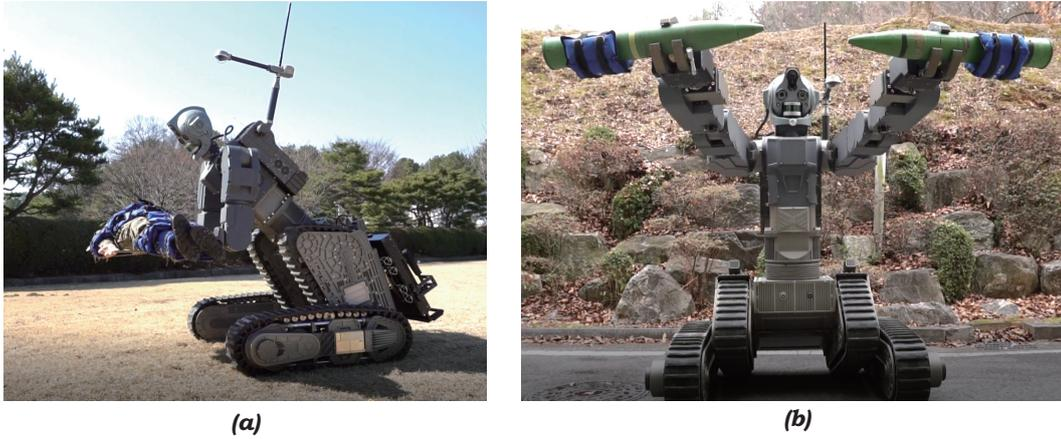
Figure 4.4: Maximum weight lifting capacity: (a) casualty extraction (120kg) (b) explosive ordnance transportation (30kg per arm)
