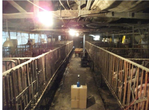
<b> Particulate matter being measured in the aisle of the pig house
