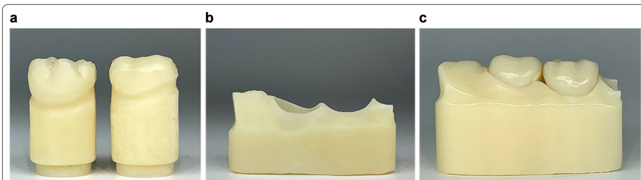
Fig. 3 Representing images of the 3D-reproduced crown dye and model base for IDBs tested. a Model, b Modelbase, c Combined model and modelbase
