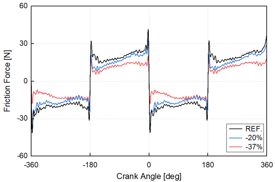
Figure 4-20. Piston friction force as OCR tension change at 60°C
