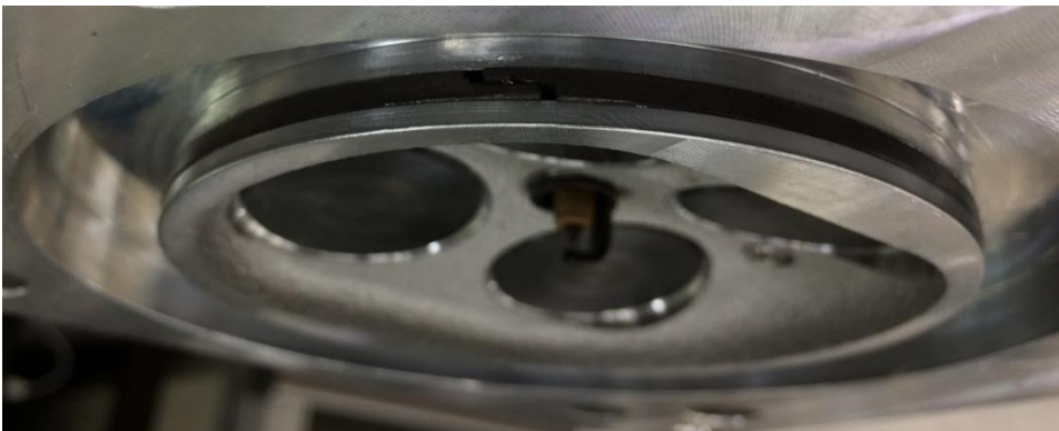
Figure 2-15. Gas seal placement in cylinder head groove
