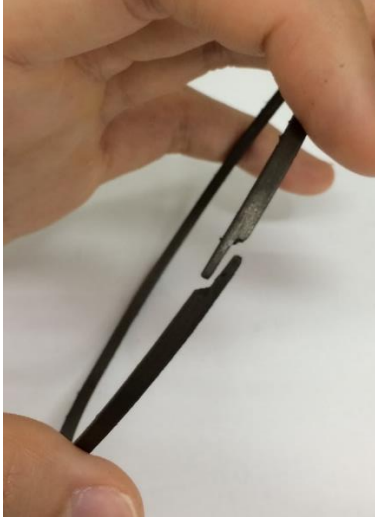
Figure 2-14. Gas seal joint shape
