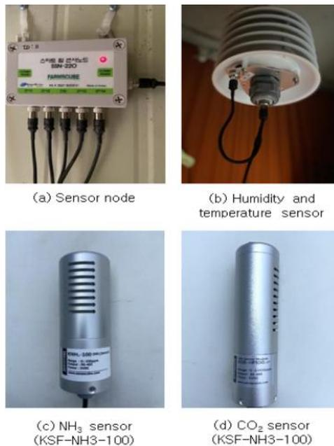
**Figure 7** Overview of sensors used in the experiment (a) Sensor node (b) Humidity and temperature sensor, (c) NH<sub>3</sub> sensor, and (d) CO<sub>2</sub> sensor (Korea Digital, South Korea)
