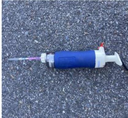
**Figure 16** Ammonia gas detector with glass tube
