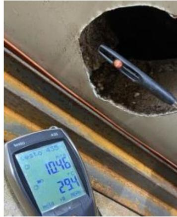
**Figure 12** Measuring air velocity at outlet
