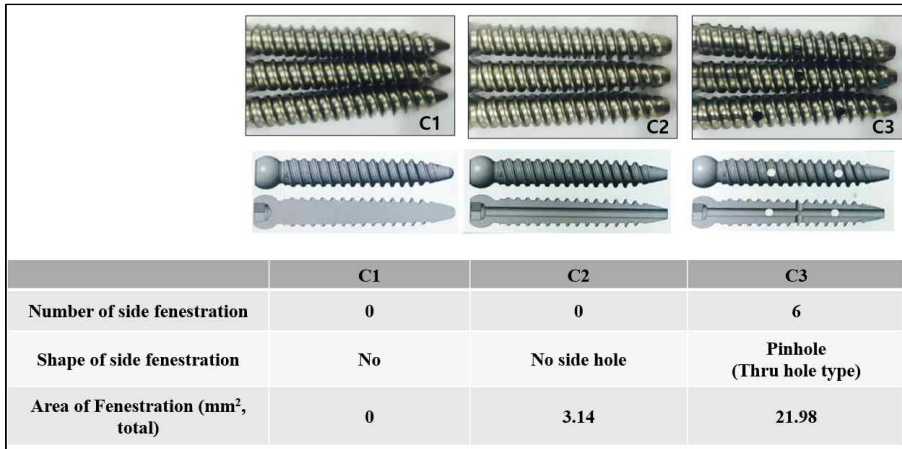
Figure 2. Comparing the characteristics of control group screws with photographs and cross-sections. The screw without fenestration, the prototype of the pedicle screw, was defined as C1, the screw with an end hole at the tip of the screw was defined as C2, and the screw with six thru-hole-shaped side pinholes was defined as C3.
