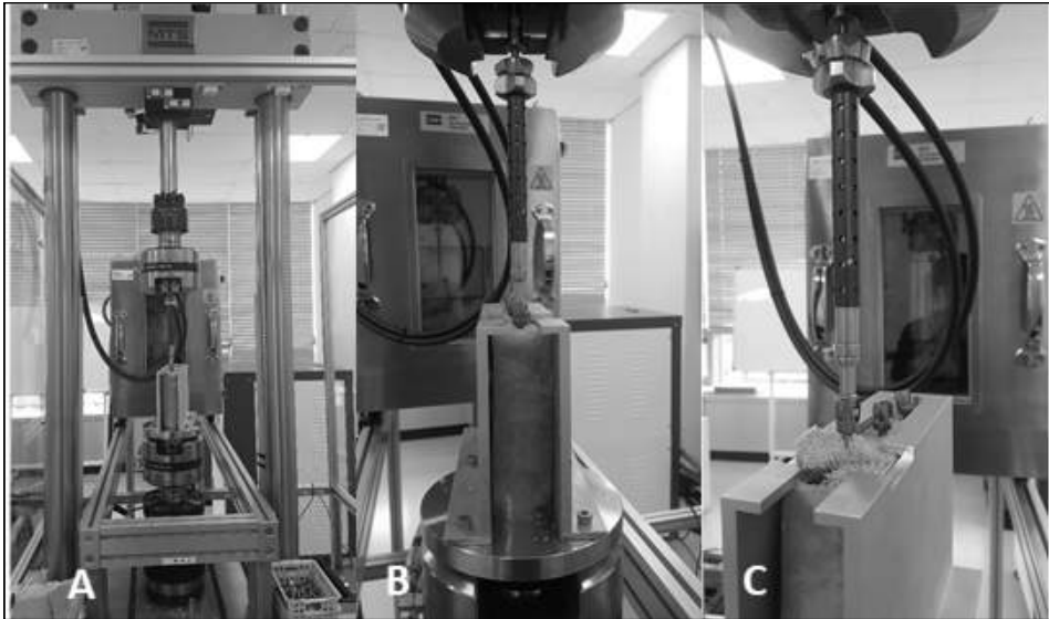
Figure 7. Pull-out strength test using the MTS system (Bionix 858, MTS Systems Corp., MN, USA).(A) The specimen was mounted on the test jig of a universal material testing machine.(B) The test jig fastened to the upper head of the inserted pedicle screw was tensioned at a speed of 5 mm/min until the pedicle screw inserted into the test block was separated.(C)
