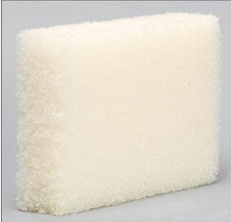
Figure 6. Synthetic bone (model #1522-505; Pacific Research Laboratory Inc., Vashon Island, WA, USA) made from polyurethane foam was shown. It was supplied as a rectangular feature (test block) with dimensions of 13 cm × 18 cm × 4 cm; the material was an open-cell rigid polyurethane foam with a density of 0.09 g/cm 3 and grade 7.5 pounds per cubic foot (pcf).
