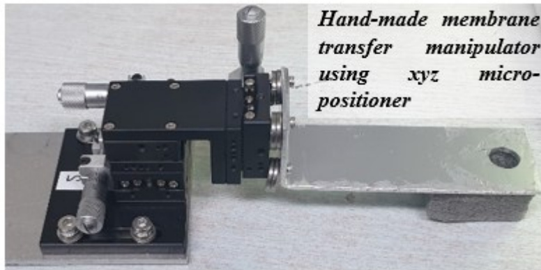
Figure A.6 Photograph of hand-made membrane transferring manipulator attached to the xyz micro positioner.
