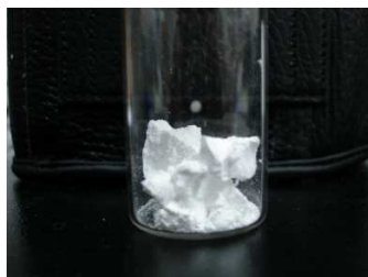
Figure 2.17: White Gd-TMHA salt the following filtration with 0.2 \mu\text{m} pore size Te on the membrane filter.
