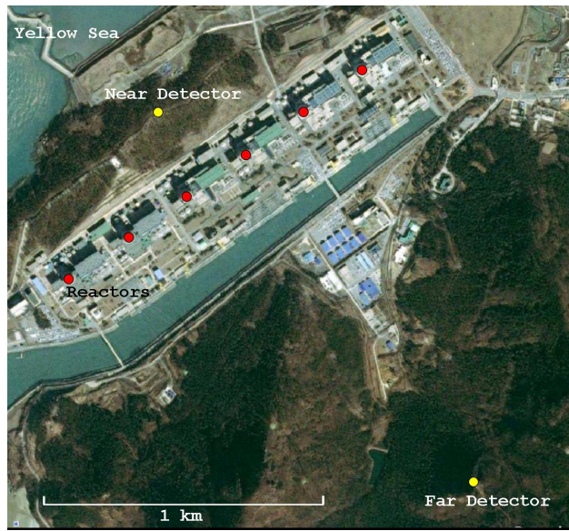
Figure 2.3: The Arrangement of the RENO experimental site. The red dots are reactors, and the yellow dots are detectors. Six reactors are equally spaced at approximately 1280 m distances. ND and FD are located at a distance of 290 m and 1380 m from the center of the reactor array, respectively. This picture was taken from Google Earth™ and was copyrighted therein. © 2015 Google, DigitalGlobe
