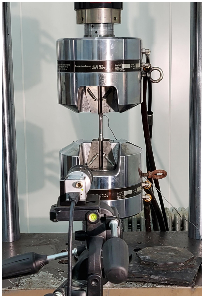
Figure 2.5 Projectile tensile test setup
