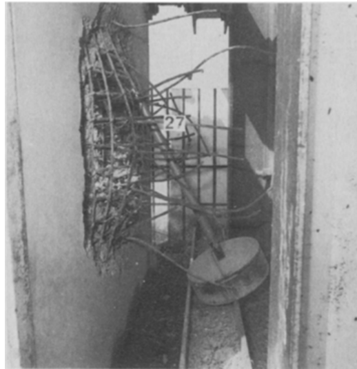
Figure 4.3 Perforation of RC panel (Berriaud (1978))
