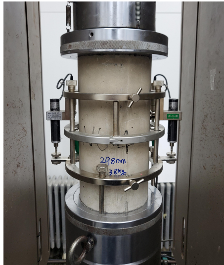
Figure 2.1 Concrete compressive test setup
