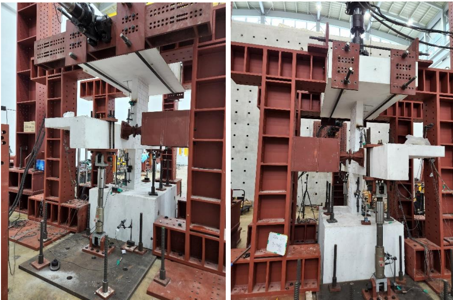
Figure 4-19 Test setup in Out-of-plane
