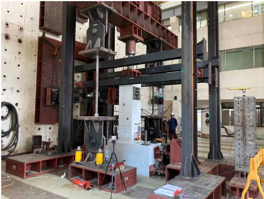
Figure 4-9 Test setup of column tests
