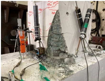
(c) Sleeve cover spalling of a tensile side ( \delta = 2.75\% )
