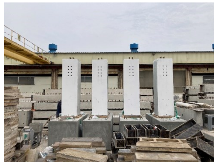
(b) Column-base assembling and manufacturing mold
