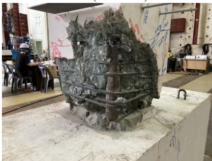
(e) Concrete cover removal after test
