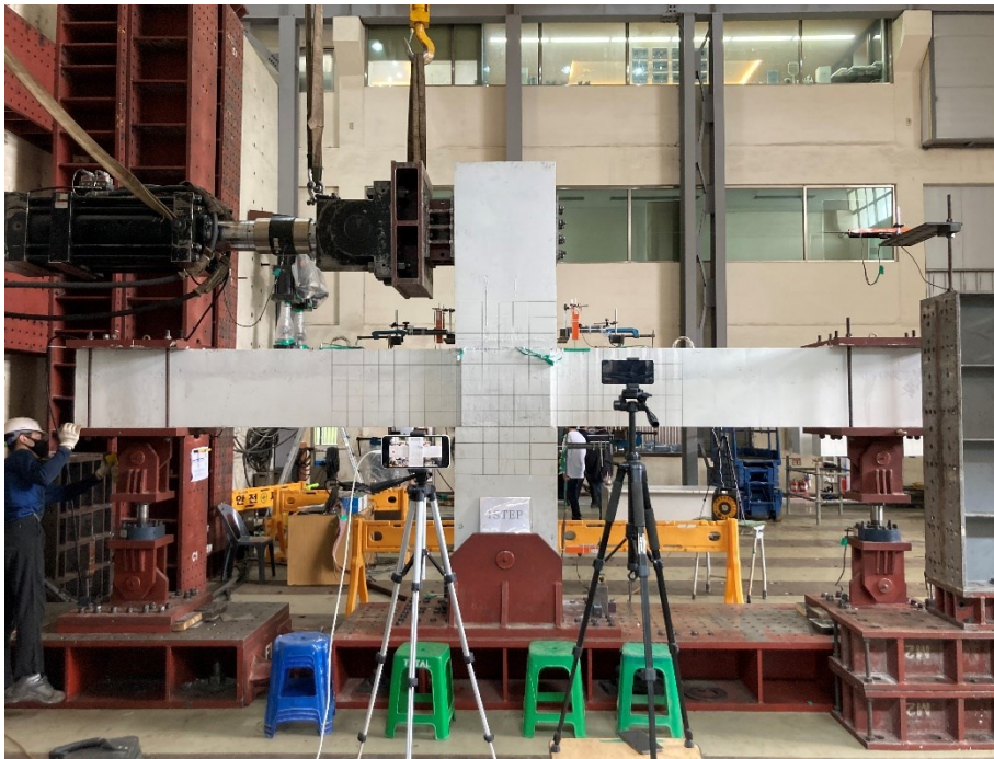
Figure 5-8 Test setup of the beam-column connection tests
