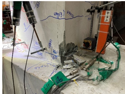
(b) Concrete cover vertical cracking
