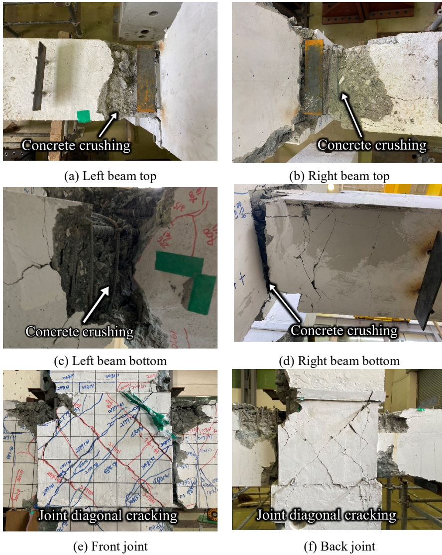
Figure 5-15 J-G1 detailed failure pictures
