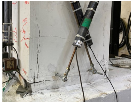
(b) Concrete cover vertical cracking
