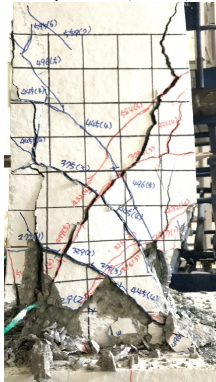
(e) Final failure (front) ( \delta = 3.5\% )
