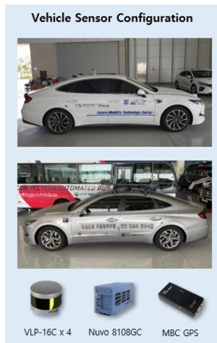
Figure 3.6. Driving data collection vehicle sensor configuration
