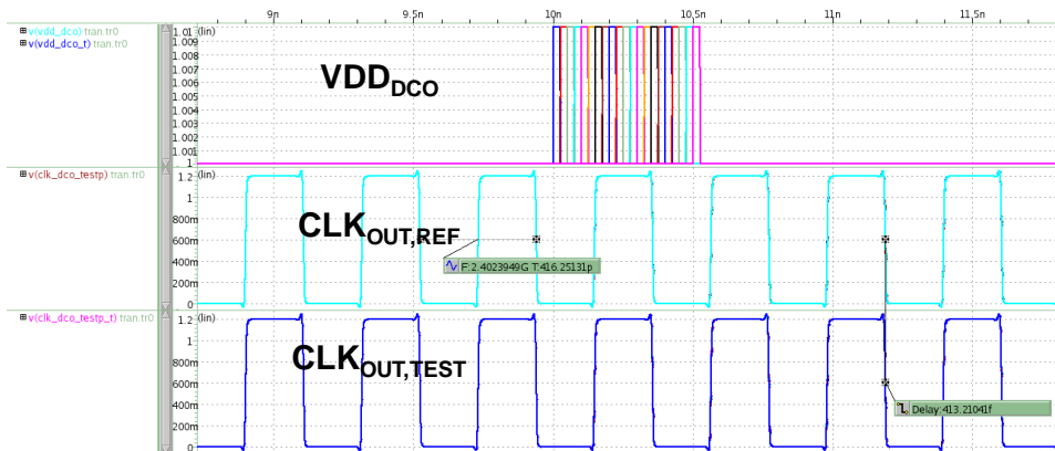
Fig. 3.2 Simulation method of the impulse voltage injection to the supply node.
