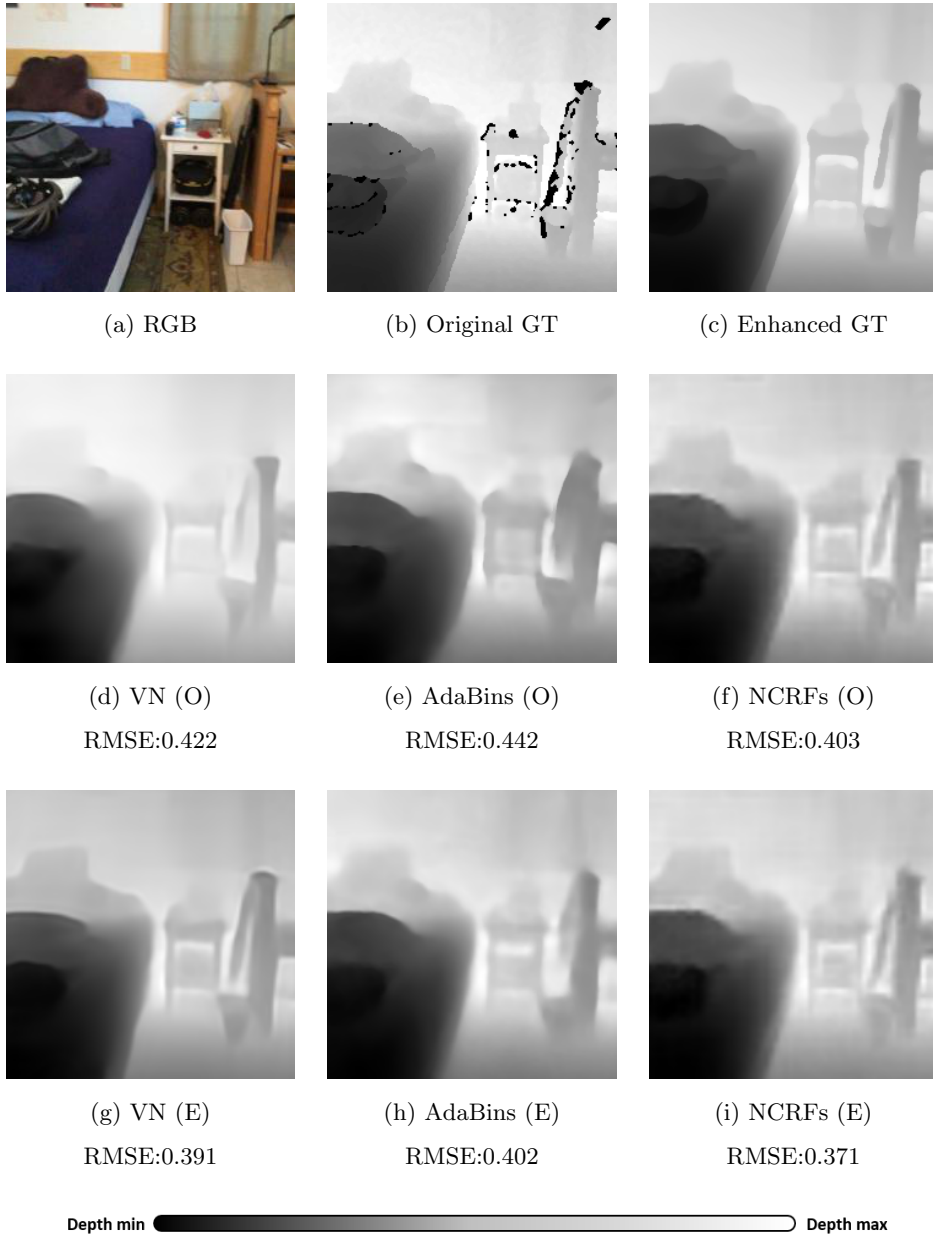
Figure 5.16: Qualitative comparisons of the original and enhanced ground-truth depth dataset. The depth estimation results trained by using the original dataset are written as “O”, and the results by enhanced ground-truth dataset are written as “E” in the parentheses following each method.
