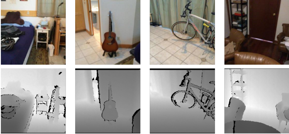
Figure 1.2: RGB-D pairs captured from commercial depth sensor. Top row: RGB images; bottom row: corresponding depth images. The depth images contain noise and missing values.
