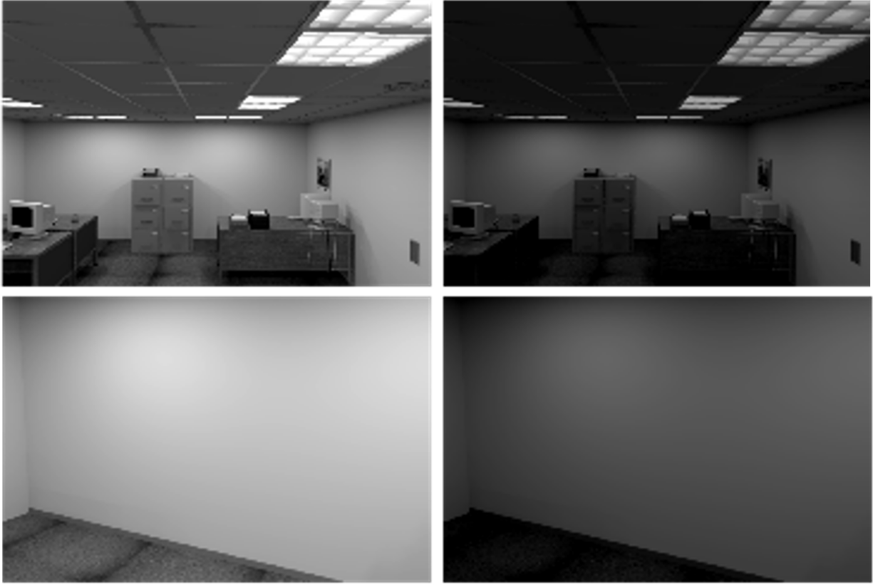
Figure 4.2: Representative scenes of the ICL-NUIM datasets (left figures), and simulated brightness changes (right figures)[3].
