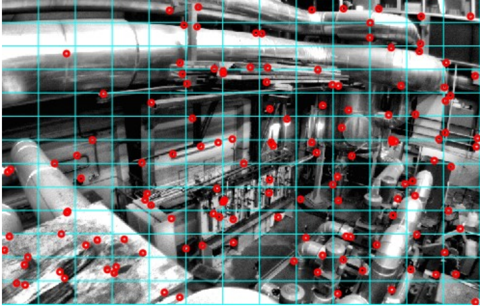
Figure 2.15: Feature bucketing strategy to maintain the number of edge and point pixels
