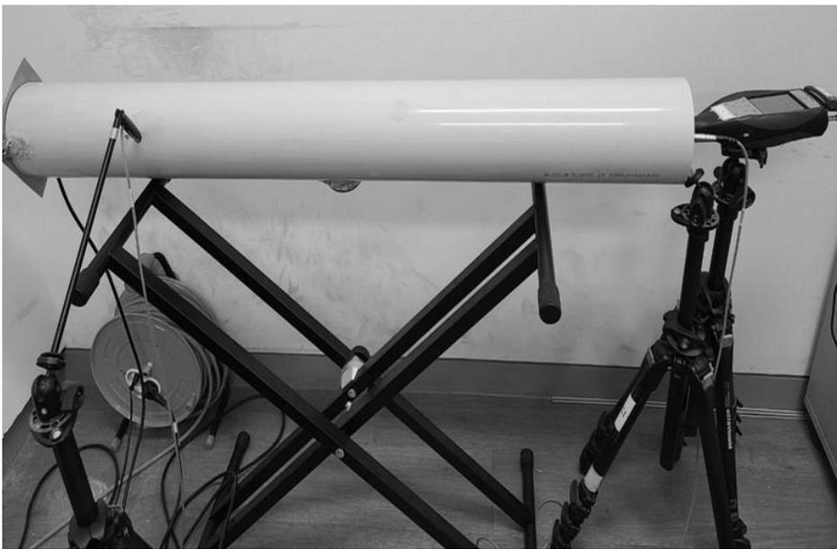
(b) Duct ANC experimental setup
