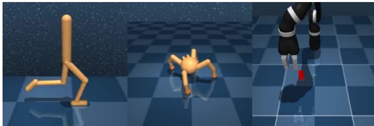
Figure 4.1: Continuous control environments from DeepMind Control Suite. Left: Walker, center: Quadruped, right: Jaco arm.
