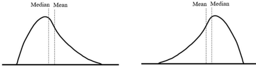
Figure 5: Skewness (left: when the skewness value is positive, right: when the skewness value is negative)
