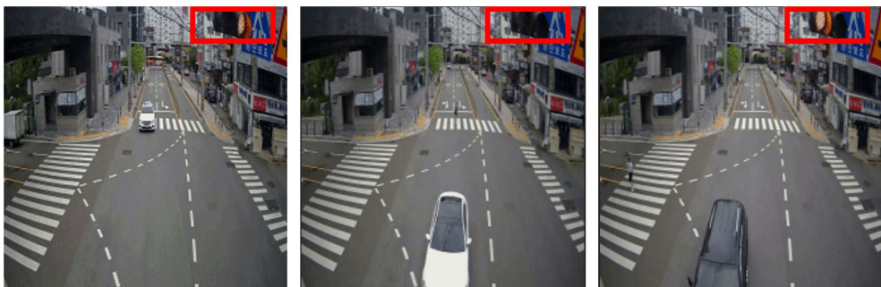
Figure 3.2: The constant change of traffic signs will cause false-positive when using subtraction-based motion detector.
