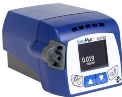
Figure 2. A real-time laser photometer (SidePak AM520, TSI, MN, USA).
