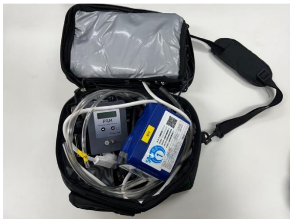
Figure 1. A packaged bag with real-time monitors of PM 2.5 , O 3 , temperature, and RH.
