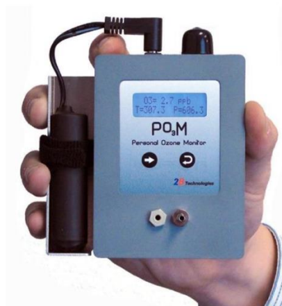
Figure 3. A miniaturized O 3 monitor (Personal Ozone Monitor, 2B technologies, USA).
