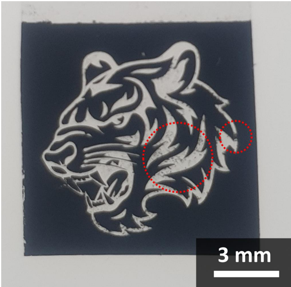
Figure 3.1. Photograph of the graphical pattern of CNT/paraffin composite with CNT residues.
