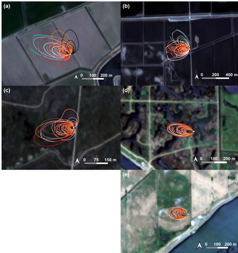
Figure S4.8 Examples of daily eddy covariance (EC) footprints at sites (a) US-Bi1 (Alfalfa), (b) US-Bi2 (Corn), (c) US-Tw4 (Freshwater wetland), (d) US-Myb (Palustrine wetland), and (e) US-Snf (Pasture) from July 1–10 (colored lines at each date), 2018 (a–c) and 2019 (d–e). Contour lines delineate footprints within which (a–c) 50–90% and (d) 50–80% of the cumulative flux originated. Image source: red–green–black (RGB) Planet Fusion surface reflectance product (projection, WGS84/UTM zone 10N) for (a–c) July 1, 2018, and (d–e) July 1, 2019.
