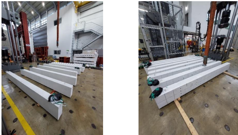
Figure 3.17 Grid work on the surface of RC beams
