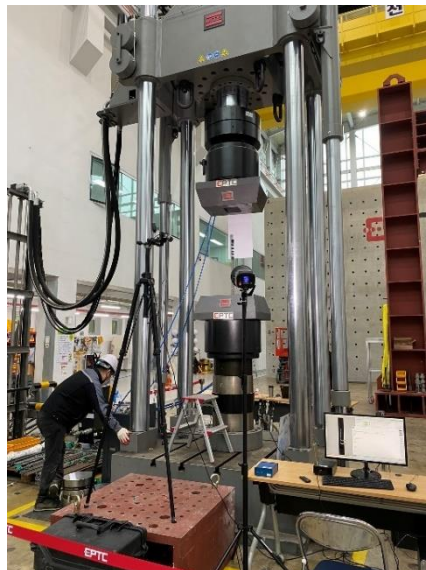
Figure 3.5 Uniaxial tension test of reinforcing steel bars
