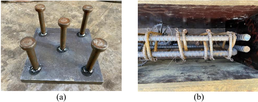
Figure 3.8 Reinforcement on the support of beams: (a) Steel plate; (b) Steel plate in RC beams
