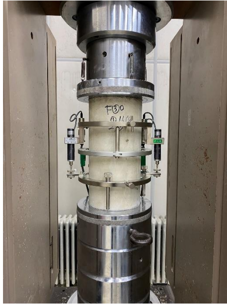
Figure 3.4 Compression test of concrete cylinder
