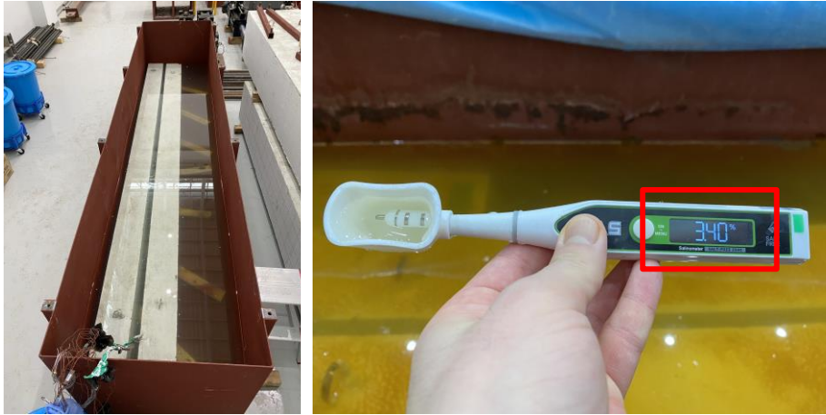
Figure 3.10 Seawater saturation of RC beams
