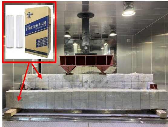
Figure 3.20 Actual test setup of RC beams in freeze-thaw cycles
