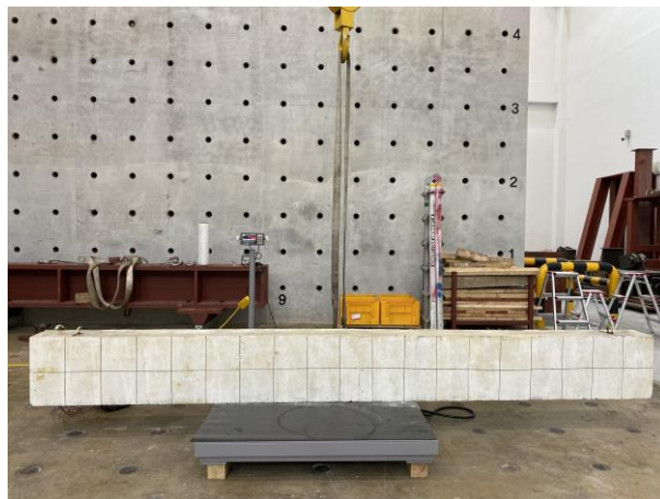
Figure 3.11 Weighting of seawater-immersed RC beams
