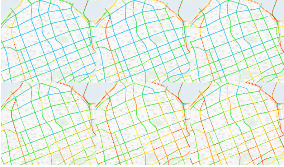
Figure 4.9: Propagation of speed reduction through an interrupted flow. Each subfigure's time step starts from 6:00 am to 8:00 30 min interval
