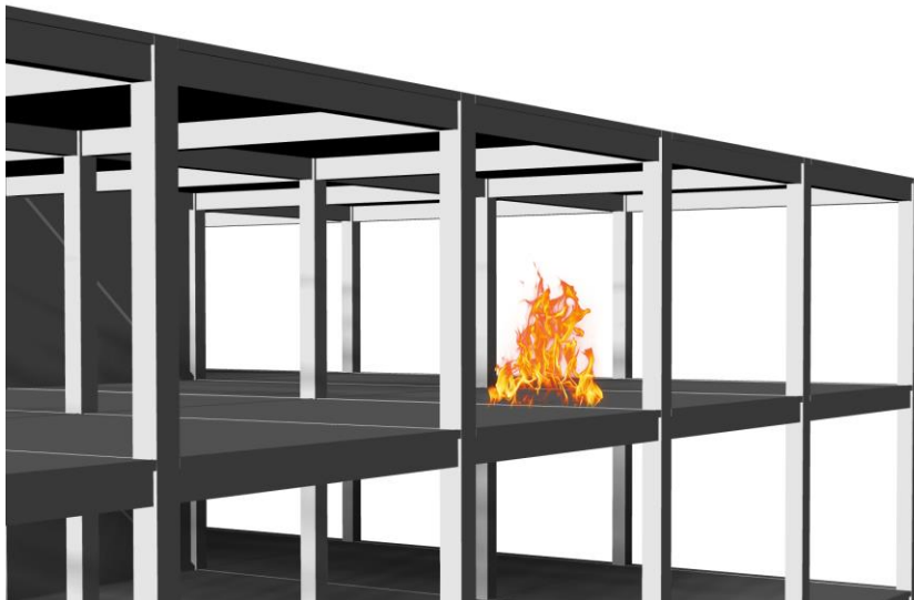
Figure 1.1 Uneven heating in structure
