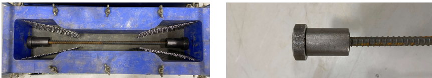
Figure 1-8 Wire mesh and anchor head installed in the specimen
