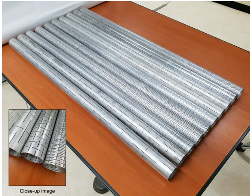
Figure 3-8. Auxetic meta-tube specimens. The auxetic meta-tubes are fabricated by high-resolution laser cutting.
