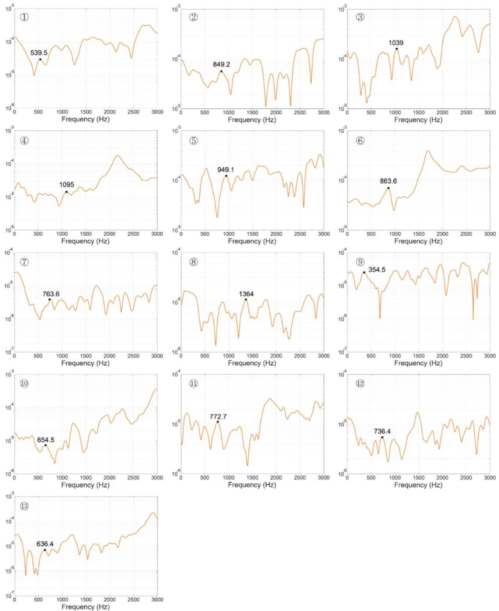
Figure A-2. Frequency Response Functions (FRFs) of the auxetic tubes imposed a torsional impact force. The marked frequencies indicate the first mode torsional natural frequencies of the tubes.
