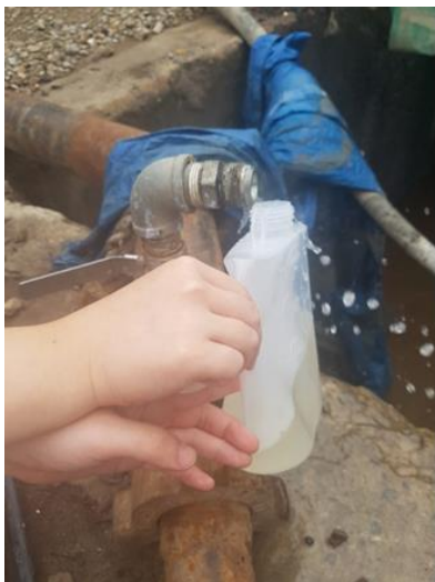
Fig. A2. Sampling injection and flowback water samples from geothermal system.
