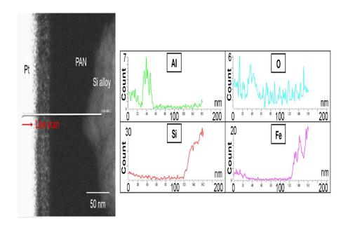
Figure 2.2. TEM-EDS line scan of Al<sub>2</sub>O<sub>3</sub>-coated anode: 50 W, 1 min.
