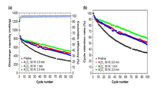
Figure 2.3. (a) Discharge capacity of Pristine and Al<sub>2</sub>O<sub>3</sub>-coated anodes.
