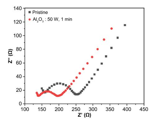
Figure 2.7. EIS results of the pristine and  $Al_2O_3$ -coated anodes: 50 W, 1 min at 100 cycles.
