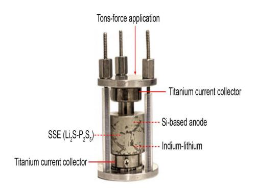
Figure 2.1. Assembly of the polyetheretherketone split cell.
