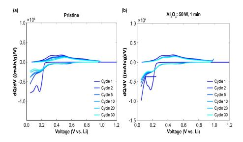
Figure 2.5. Differential capacity of the (a) pristine and (b)  $Al_2O_3$ -coated anodes: 50 W, 1 min.
