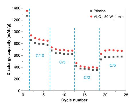
Figure 2.4. Rate capability test of the Pristine and  $Al_2O_3$ -coated anodes: 50 W, 1 min.
