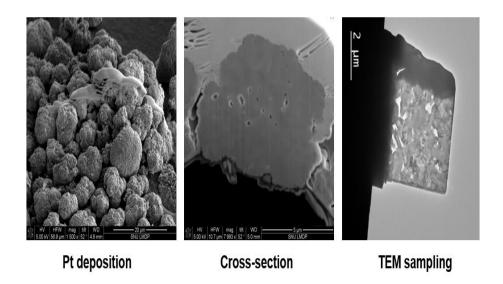
Figure 1.2. Sample preparation process for transmission electron microscopy (TEM) using FIB-SEM.
