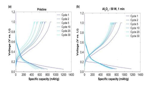
Figure 2.6. Voltage profile of the (a) pristine and (b)  $Al_2O_3$ -coated anodes: 50 W, 1 min.
